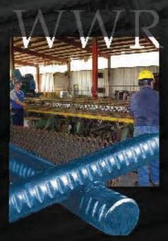
Machine Resistance Welding – Pressure and heat fuse the intersecting wires into a homogeneous section and fix all wires in their proper position. Visit www.insteel.com for more details.
