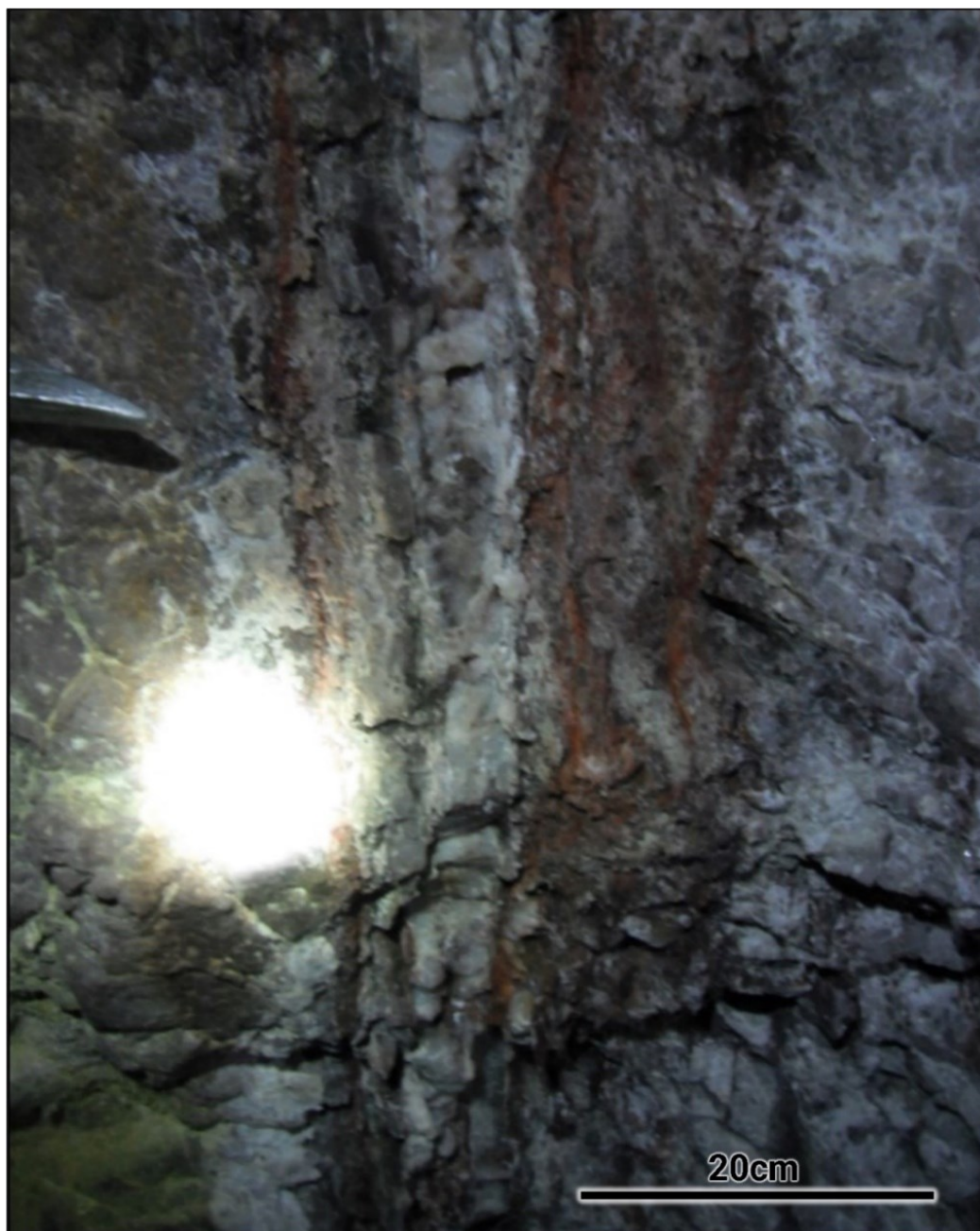
Figure 6-7: Laminated (Banded) Vein Style Mineralization Along Las Chispas Vein, Tip of Rock Hammer Shown on Upper Left (Near SilverCrest Sample 2277908, 1.04 g/t Au and 197 g/t Ag over 1.33 m)
