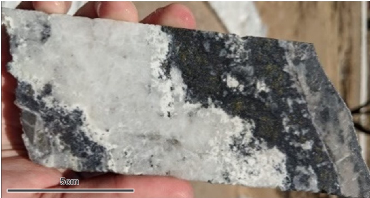
Figure 6-22: Drill Hole BAN18-10, From 93.0 to 95.5 m Grading 61.36 g/t Au and 2,834 g/t Ag with Visible Argentite, Pyrargyrite, Electrum, Native Silver, and Native Gold
