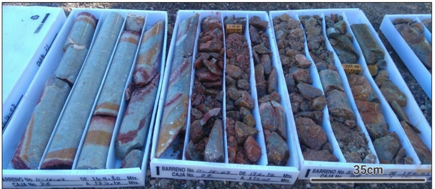
Figure 6-34: William Tell Vein, Drill Hole LC16-03, from 172 to 176 m, 4 m (1.5 m True Thickness) Grading 2.03 g/t Au and 683 g/t Ag
