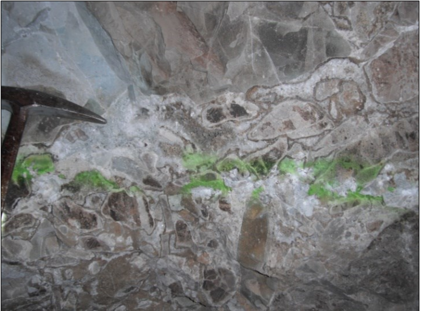
Figure 6-8: Breccia Style Mineralization Along Las Chispas Vein (Base of Las Chispas Gallery near SilverCrest Sample 617179 2.34 g/t Au and 344 g/t Ag)
