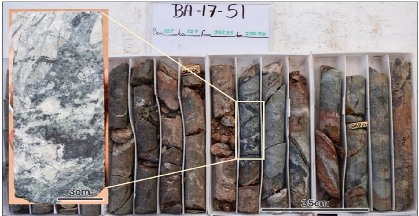
Figure 6-18: Drill Hole BA17-51 (Discovery Hole for Area 51 Zone); from 265.9 to 269.2 m, 3.3 m (3.1 m True Thickness) Grading 40.45 g/t Au and 5,375 g/t Ag, with Hematite Breccias, Coarse Banded Argentite, Native Silver, Electrum, and Native Gold.
