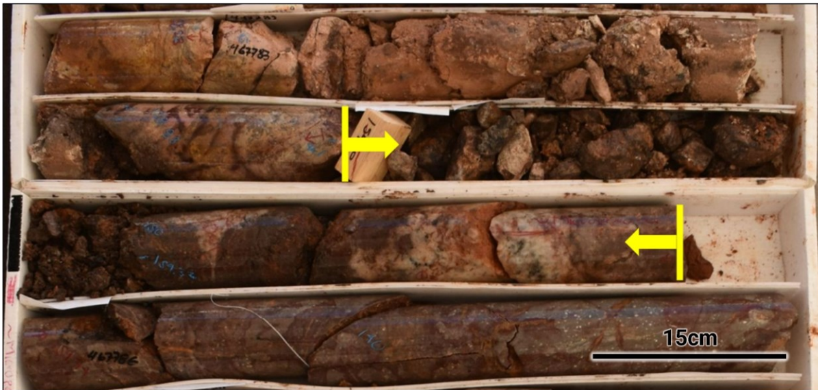
Figure 6-26: Drill Hole BAS22-209, from 159.00 to 160.45 m at 1.0 m (True Thickness) Grading 38.12 g/t Au and 165.0 g/t Ag
