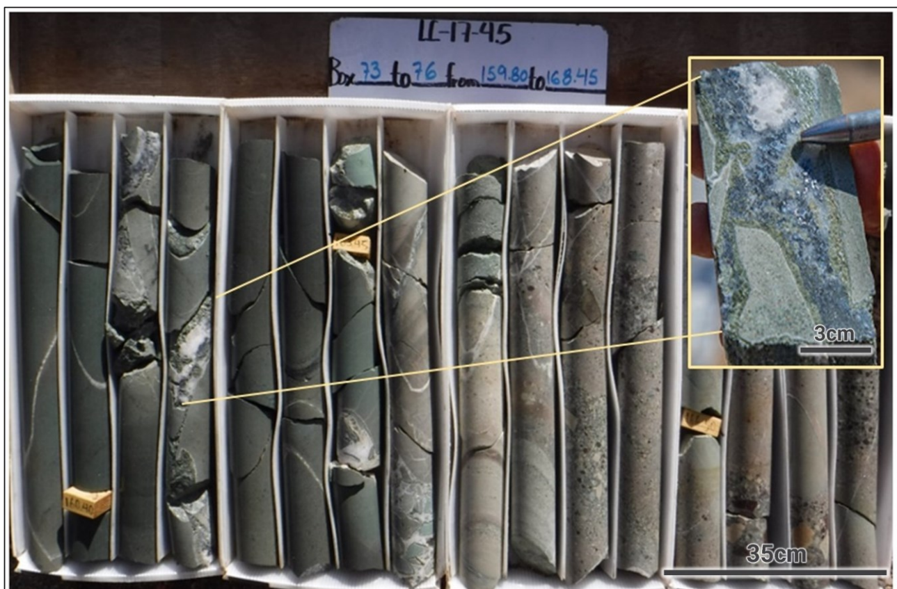
Figure 6-29: Drill Hole LC17-45; from 159.6 to 161.9 m at 2.3 m (1.9 m True Thickness) Grading 50.56 g/t Au and 5,019 g/t Ag with Coarse Argentite and Electrum
