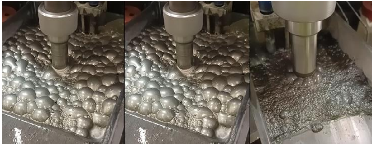
Figure 10-8: Open-Circuit Cleaner Flotation Concentrate
