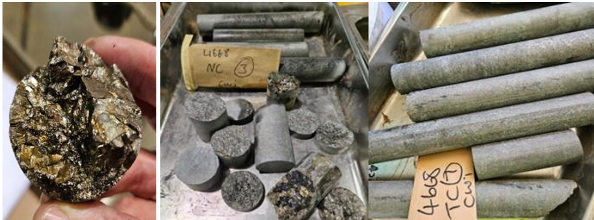
Figure 10-2: Example of Concentrator Metallurgical Testwork Drill Core Intervals
