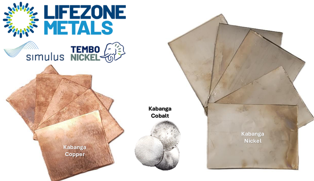
Figure 3: Nickel, copper and cobalt samples produced by Hydromet from Kabanga source material through pilot test work completed at Lifezone’s laboratory in Perth, Australia.
