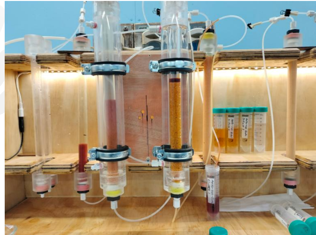
Continuous precious metals refinery test work at Lifzone’s Simulus Laboratories
