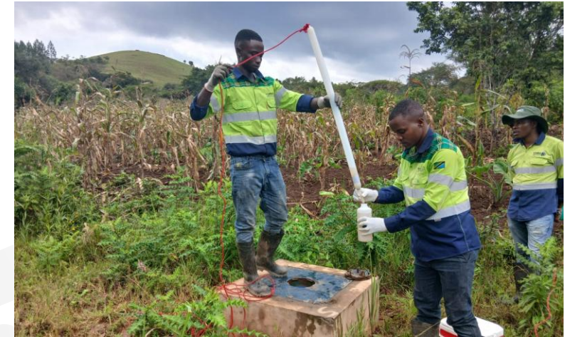
Production water borehole drilling at Kabanga Site, 132m deep, providing a yield of 28,000 L/H
