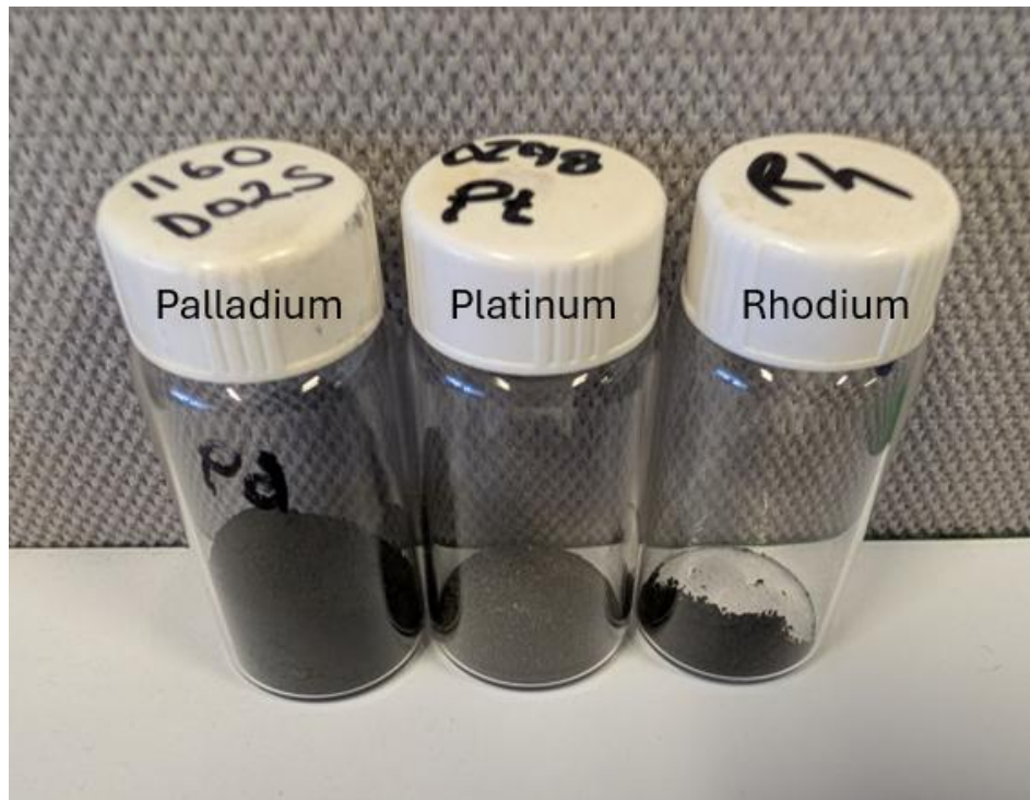
Figure 1: Platinum, palladium and rhodium samples produced by Lifezone’s Hydromet Technology from spent Autocats through pilot test work completed at Lifezone’s Simulus Laboratories in Perth, Australia.
