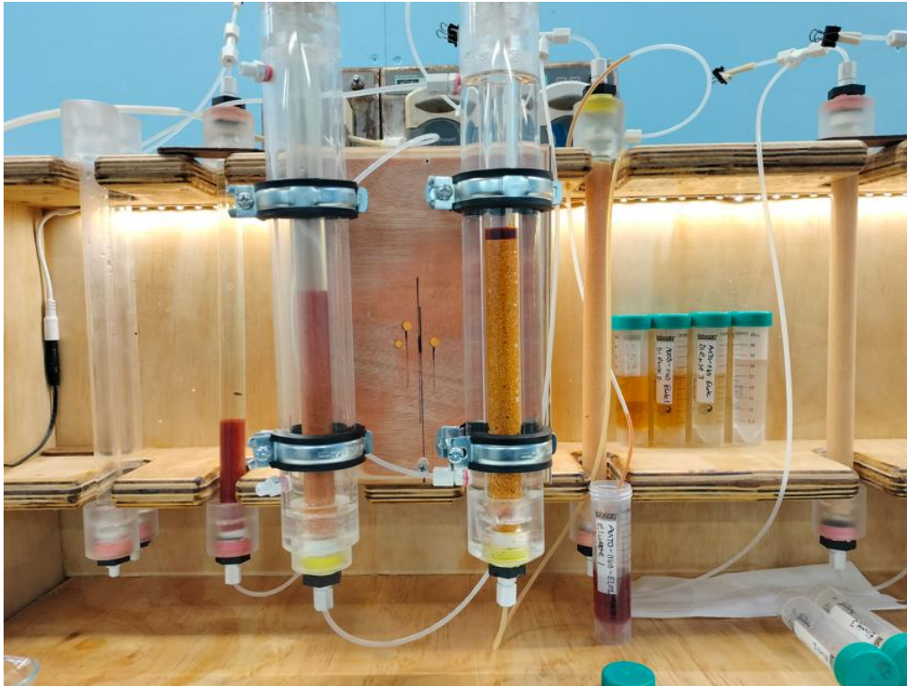
Figure 2: Continuous pilot-plant precious metals refinery test work at Lifezone's Simulus Laboratories
