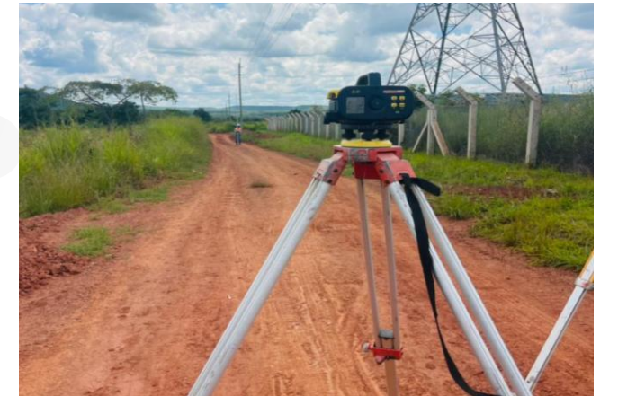
AGS leveling task through the 220Kv transmission line to determine the ground profile for angle point No.29 at Nyakanazi substation
