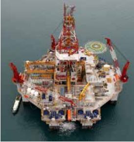
Fifth Generation Ultra-Deepwater Moored Harsh Environment Semisubmersible
